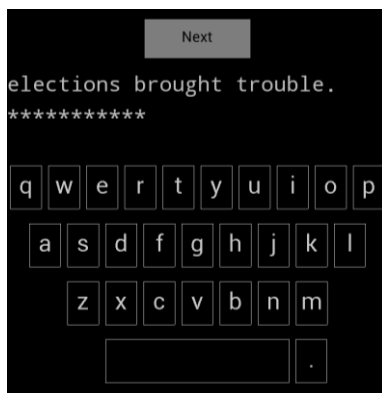
Figure 2. The WOZ keyboard for data collection, which was designed to capture fundamental text entry behaviors.
