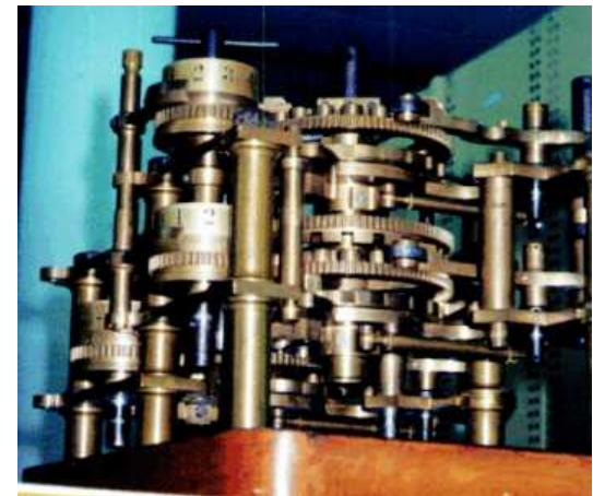
fragment made by H.P.Babbage from parts of Difference Engine No.1
