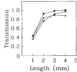
Fig. 2. Transmission coefficients of nominally  $0.5^\circ$  S-shaped bends, including cosine-generated curve (dot), two-arc design (triangle), and sine-generated curve (square) versus the length of bends.
