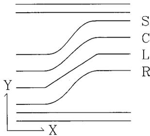
Fig. 1. Mask patterns of S-shaped bend designs. They are shown with an aspect ratio of 1:20. Four designs, including, two arcs (*R*), two arcs with a connecting straight guide (*L*), cosine-generated curve (*C*), and sine-generated curve (*S*) are used. The lateral offset is  $364 \mu\text{m}$ . The length is 12 mm. Straight waveguides are included for calibration.
