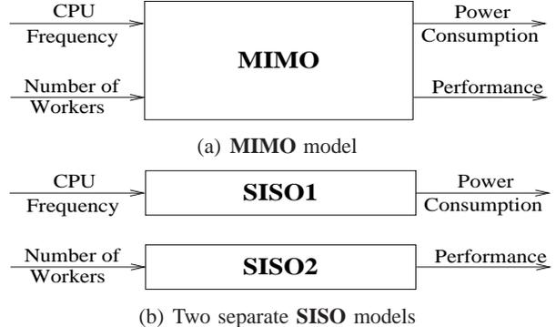
Figure 2. Our MIMO model and two-SISO models
