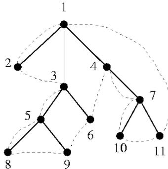
The optimum traveling salesman tour is at most twice the length of the minimum spanning tree.
