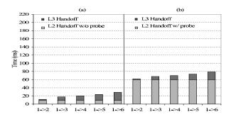
Figure 5. Handoff latencies for *iMesh* using OLSR routing with background traffic of 2.5Mbps for (a) without probing and (b) with probing on a single channel.
