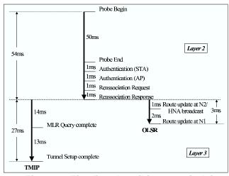
Figure 2. Timeline describing a typical fast one-hop handoff from N1 to N2 for a mobile station with *iMesh* running OLSR and TMIP.
