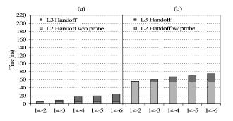
Figure 3. Handoff latencies for *iMesh* using OLSR routing with no background traffic for (a) without probing and (b) with probing on a single channel. The notation  $i \rightarrow j$  indicates hand-off from Ni directly to Nj.
