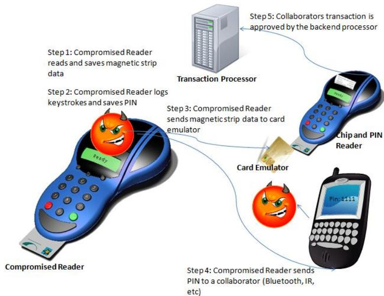
Fig. 1. A PIN and Chip based relay attack
