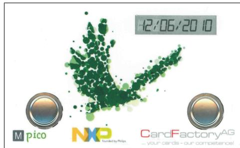
**Fig. 1.** A Display and Button Equipped RFID Tag
