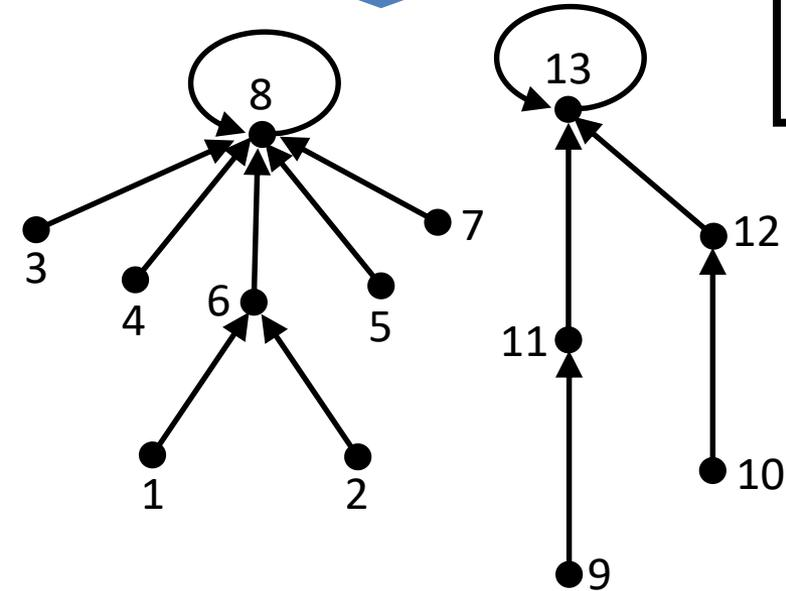
*Find-Roots* ( $n, P, S$ ) { **Input:** A forest of rooted directed trees, each with a self-loop at its root, such that each edge is specified by  $\langle v, P(v) \rangle$  for  $1 \leq v \leq n$ .
