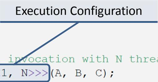
The diagram shows a box labeled "Execution Configuration" with a line pointing to the parameters of the kernel invocation: `<<<1, N>>>` in the line `VecAdd<<<1, N>>>(A, B, C);`. The parameters are also enclosed in a blue box.
