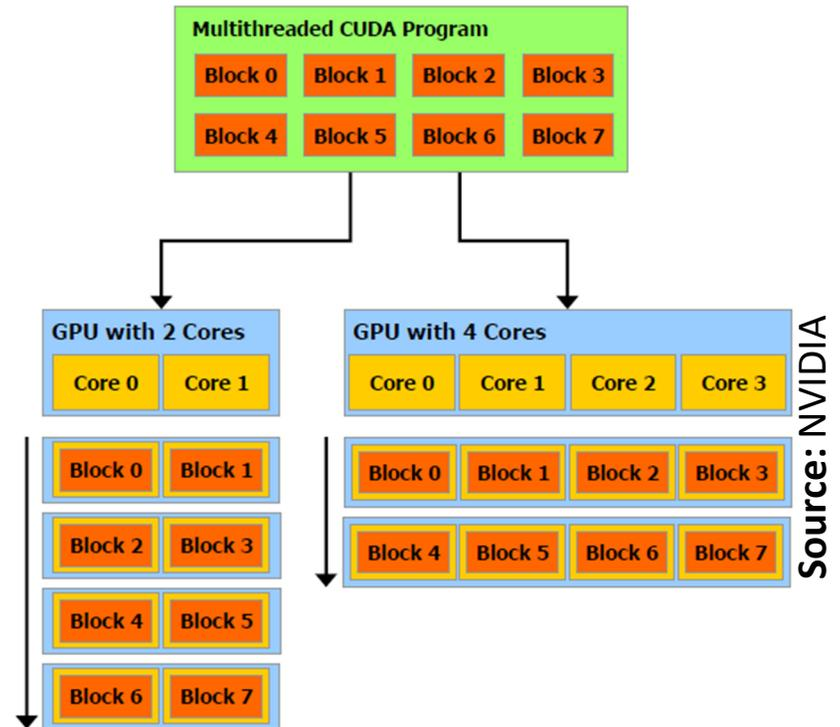
The thread blocks can be executed in any order — concurrently or sequentially — leading to automatic scalability.
