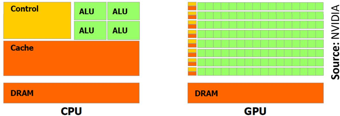
CPU's are designed for *general purpose computations* requiring sophisticated control flow and caching mechanisms.
