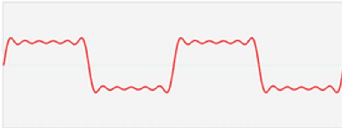
Function  $s(x)$  (in red) is a sum of six sine functions of different amplitudes and harmonically related frequencies. The Fourier transform,  $S(f)$  (in blue), which depicts amplitude vs frequency, reveals the 6 frequencies and their amplitudes.
