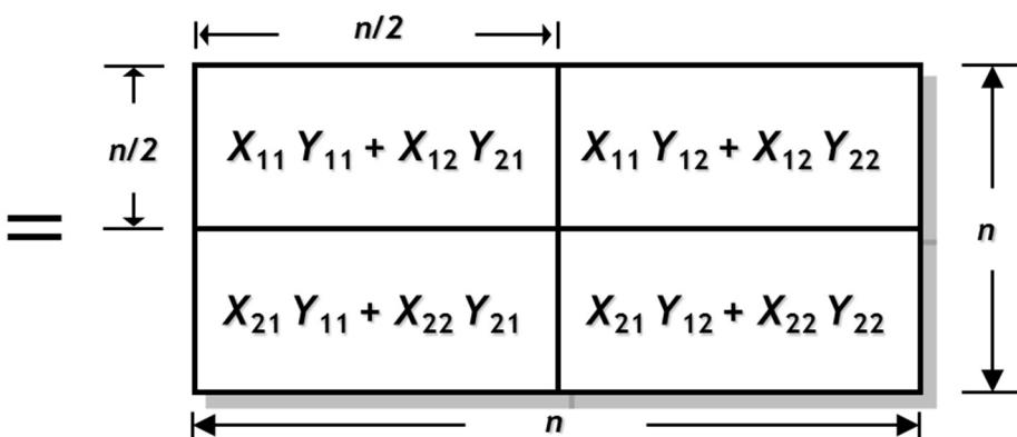
*Rec-MM (  $X, Y$  ) {  $X$  and  $Y$  are  $n \times n$  matrices,
