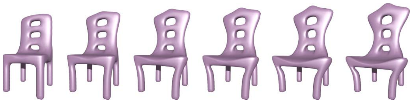
Fig. 12. A new chair is designed via force-based tools. Boundary constraints were imposed on the bottom portions of the legs to fix their positions
