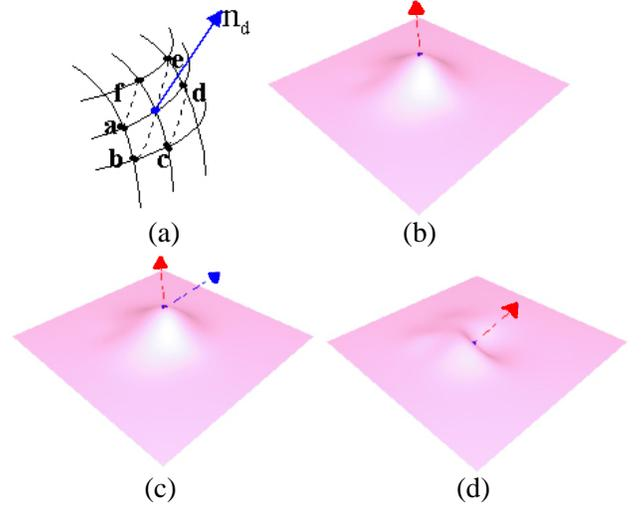
Figure 8: Normal constraint: (a) Changing the point normal will exert additional forces at the vicinity of the surface point: a,b,c,d,e,f; (b) The current normal (represented as the red arrow) is  $(-0.04, 0.07, -0.92)$ ; (c) The blue arrow represents the desired normal which is  $(0.45, -0.73, -0.52)$ , the red arrow represents the current normal; (d) The actual normal (red arrow) after surface deformation is  $(0.36, -0.64, -0.63)$ .
