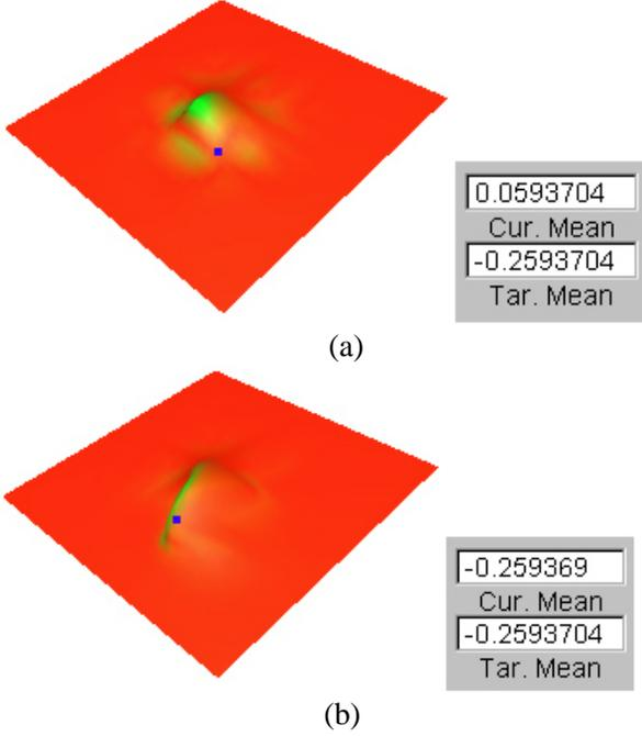
Figure 9: Curvature constraint: (a) Curvature map, green represents high curvature, red represents low curvature; the blue point is the selected point with which users want to modify its curvature, the accompanying table lists the current and target curvatures of the blue point; (b) The curvature map after users modify the blue point’s curvature; the accompanying table shows that the current curvature equals to the target curvature after surface deformation.
