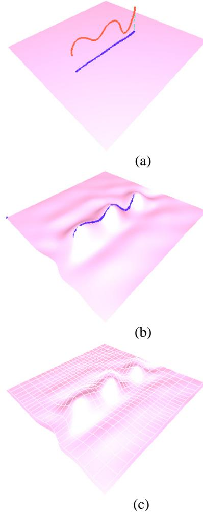
Figure 10: Curve constraint: (a) Select a spline curve tool colored in red; (b) The surface deforms in terms of the shape of the curve tool, the curve colored in blue is the corresponding curve on the D-NURBS surface; (c) The new, deformed NURBS surface satisfying the constraint of the curve feature.
