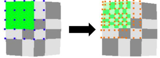
Figure 5: We subdivide the selected region (controlled by  $5 \times 5$  control points) into  $6 \times 6$  patches (controlled by  $9 \times 9$  control points) without introducing new patches in any other regions.
