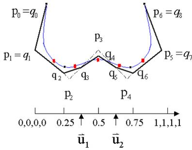
Figure 3: The new NURBS curve and its span decomposition after the insertion of two additional knots.
