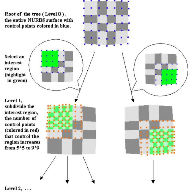
Figure 6: The D-NURBS tree and its hierarchical structure.
