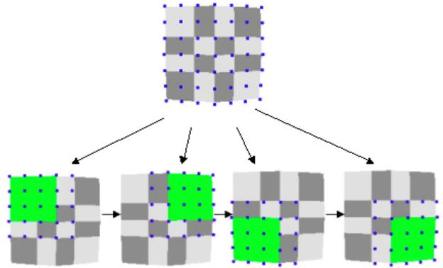
Figure 2: The NURBS surface, which consists of  $4 \times 4$  patches and controlled by  $7 \times 7$  control points (colored in blue), can be decomposed into 4 sub-regions (highlighted in green), each sub-region is controlled by  $5 \times 5$  control points.
