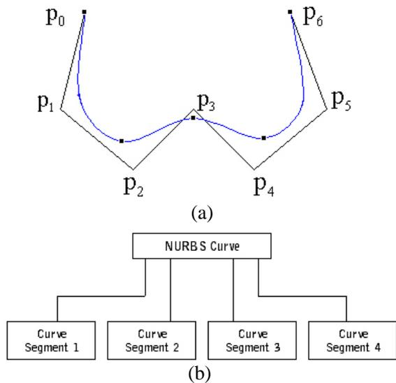
Figure 1: A NURBS curve: (a) A NURBS curve consists of 4 curve segments; (b) We consider it as a collection of 4 finite elements.
