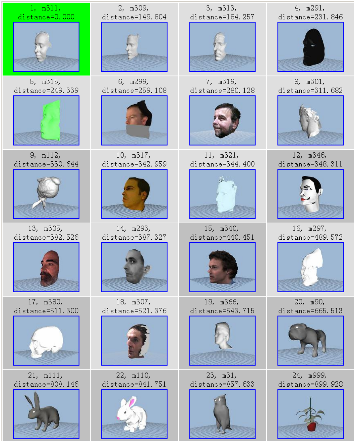
Fig 10. Another example of “partial to partial” 3D model retrieval. Note that only 40% of the spin images and point samples nearest to a point of interest of a query shape are used to match the partial shapes (also 40% of a global shape) of the database models. This is an extremely challenging task, since the expected overlap covers only 16% of the overall shape. The retrieval results are generally not very good as anticipated. However, some shapes are approximately symmetric, such as human faces. In such cases, the expected overlap is higher, and some retrieval results are reasonably good, shown in this figure.
