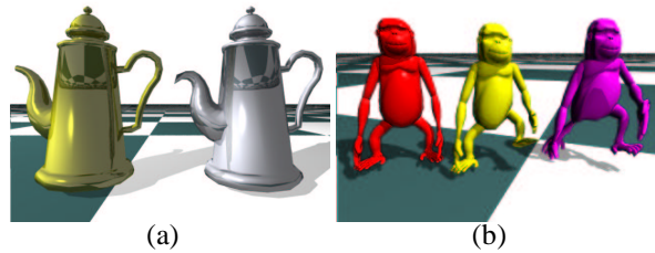
Figure 7. Direct modification of the trimmed PDE solid: (a) Directly moving a selected point on the trimmed data, on the left is the original dataset, and on the right is the modified trimmed PDE solid; (b) the deforming sequence of an trimmed object by rotating selected interior regions.
