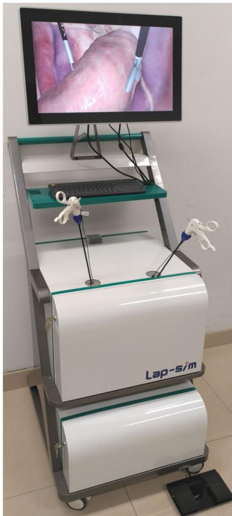
**FIGURE 3** Hardware interface of our simulator, including (from top to bottom) touch screen, keyboard, simulator case with surgery handles, and foot pedal
