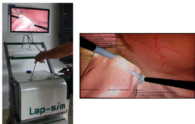
Fig. 15 Interface of our prototyped VR laparoscopic surgery simulator
