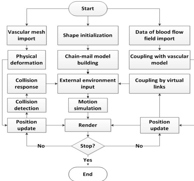
Figure 1. The flowchart of our new guidewire simulation method.
