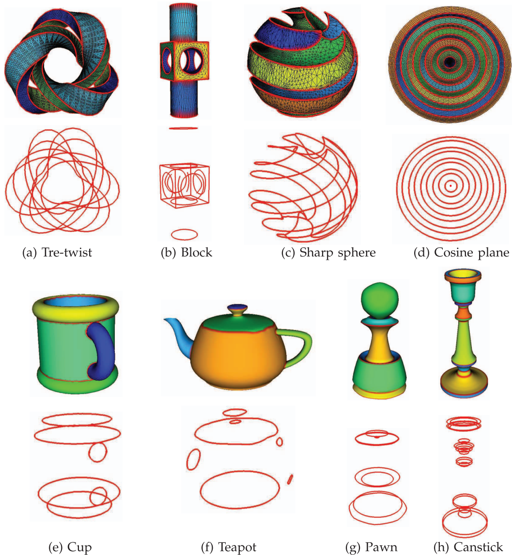
Fig. 11. More examples for man-made objects ( c_f = 0.03 , \delta_D = 0.16 ). The connected curve features are highlighted beneath the feature classification results.
