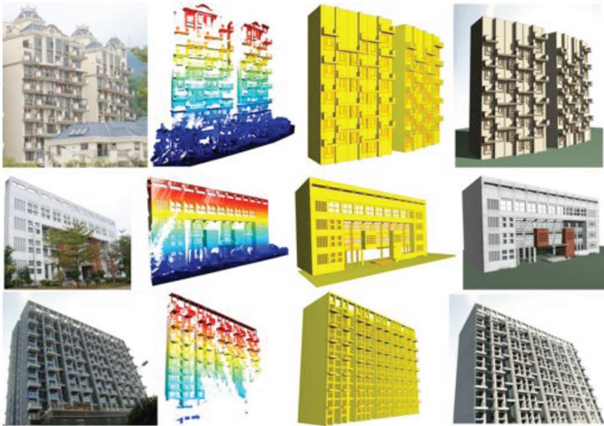
Figure 11: Additional reconstruction results using SmartBoxes. From left to right: real photograph, LiDAR scan, 3D reconstruction, and its textured version for a visual comparison with the photograph. The examples show reconstruction of complex buildings with some irregularity. Grouping and contextual force during drag-and-drop allow the reconstruction to deal with large-scale missing data (bottom row).
