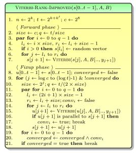
**Fig. 4.** Processor-oblivious parallel Viterbi algorithm using rank convergence.
