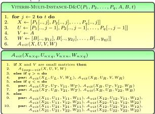
Fig. 2. Cache-efficient multi-instance Viterbi algorithm.
