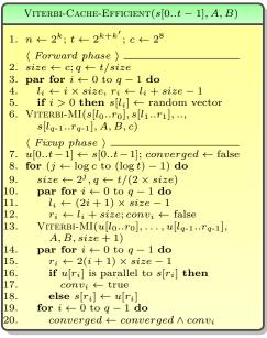
Fig. 5. An efficient cache- and processoroblivious parallel Viterbi algorithm using rank convergence. VITERBI-MI refers to VITERBI-MULTI-INSTANCE-D&C of Sec. 3.
