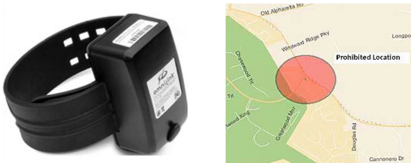
FIGURE 8.5: OmniLink's "Offender Tracking Technology" bracelet uses GPS and cell-tower location for indoor and outdoor location estimation. The ankle bracelet is shown left, and a snippet of their profile creation tool is shown right.
