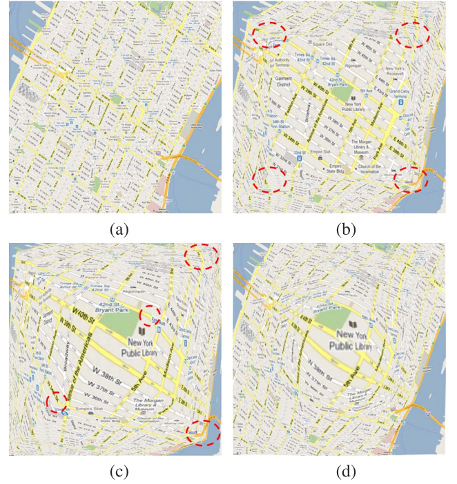
Fig. 13. Magnification results using different lenses for the NYC street map. (a) Original NYC map. Magnification results using (b) the bifocal lens, (c) the fisheye lens, and (d) our conformal magnifier. The red circles highlight the seriously distorted areas.
