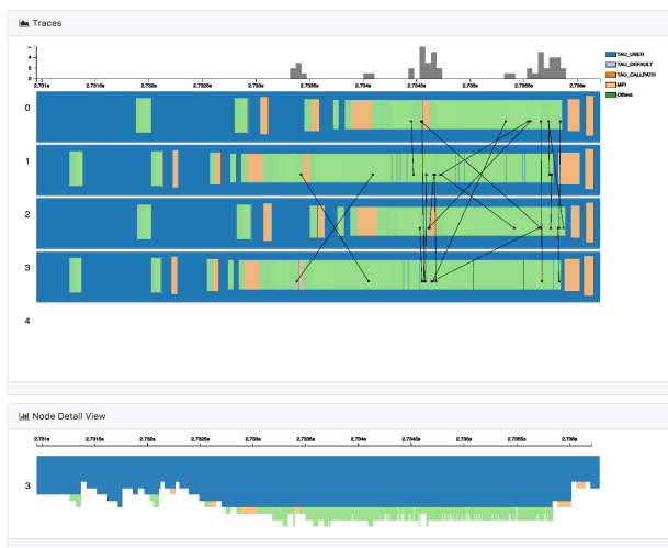
Figure 9: The node detail panel: a coarse level of selected timeline of node 3 is shown. The trace panel and the node detail panel are aligned along the time axis.
