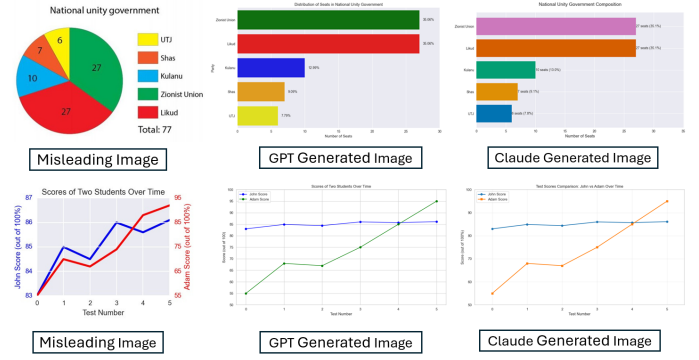
Fig. 4: Comparison of original misleading visualizations and MisVisFix-generated corrections. Top: Pie chart with too many similar-colored segments converted to sorted bar chart after detecting inappropriate chart type, indistinguishable colors, and missing units. Bottom: Line chart with dual y-axes causing data misrepresentation replaced with single-axis line charts after identifying dual axis issues, data magnitude differences, and misrepresentation problems. Both examples show conversion to clearer chart formats that reduce misinterpretation and improve data comprehension.
