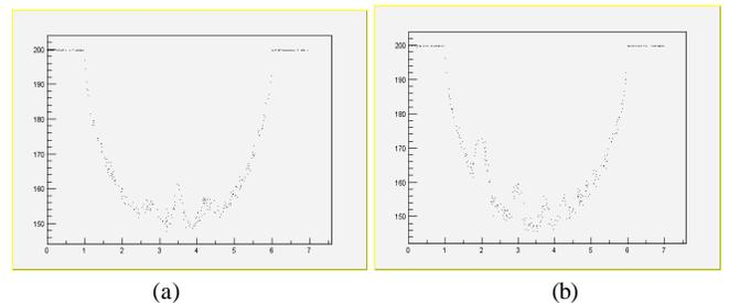
Fig. 4. Residual energy versus entry position at different views: (a) view angle  $0^\circ$ , (b) view angle  $90^\circ$ . Some phantom structures are already reflected in these one-view profiles.
