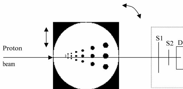
Fig. 1. Schematic diagram of a conceptual pCT system. The proton pencil beam and detectors remain stationary while the object moves and rotates. The detection part includes two position sensitive silicon detectors (S1 and S2), and a scintillation detector (D) to measure the residual proton energy.
