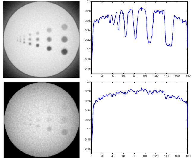
Fig. 7. Reconstructed images and horizontal profiles for different contrast phantom simulations. (Top row: high contrast, middle row: medium contrast; bottom row: low contrast).
