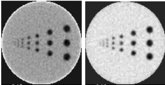
Fig. 6. Reconstructed image using interpolation without (left) and with (right) estimated path  $L'$ .
