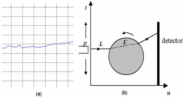
Fig. 2. The “path” of the proton inside the object. (a) The real proton path inside the object is zigzag. (b) Since both the position and direction of the exit proton can be measured and the entry direction is known, the cross-points of the proton beam with the object boundary can be obtained. The proton path,  $L'$ , is then approximated by the dashed line.
