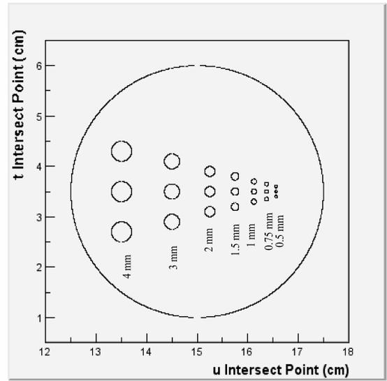
Fig. 3. Lab reference system for the simulations. The phantom is centered at (15, 3.5), the protons arrive along  $u$  direction at plane  $u=0$  cm. The detector is at  $u=30$  cm.
