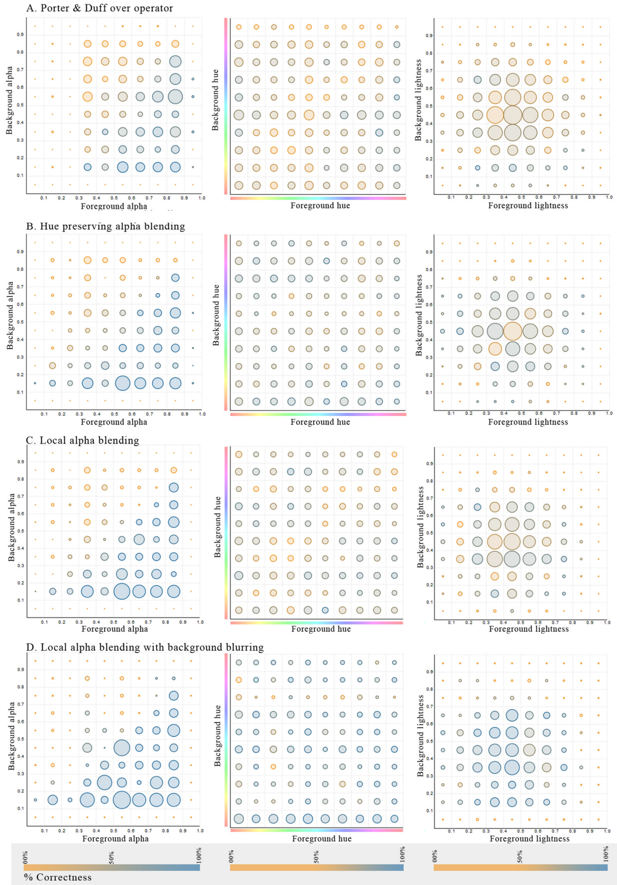
Figure 6. Visualization to evaluate the performance of different blending algorithms for transparency perception. For each of the algorithms we produce three scatterplots concerning variation in alpha value, hue and lightness of the colors. Each of the plots shows the number of data points collected and the correctness for different foreground and background combinations. The color of the circle represents the correctness for that particular combination. The size of each circle is proportional to the data point count.
