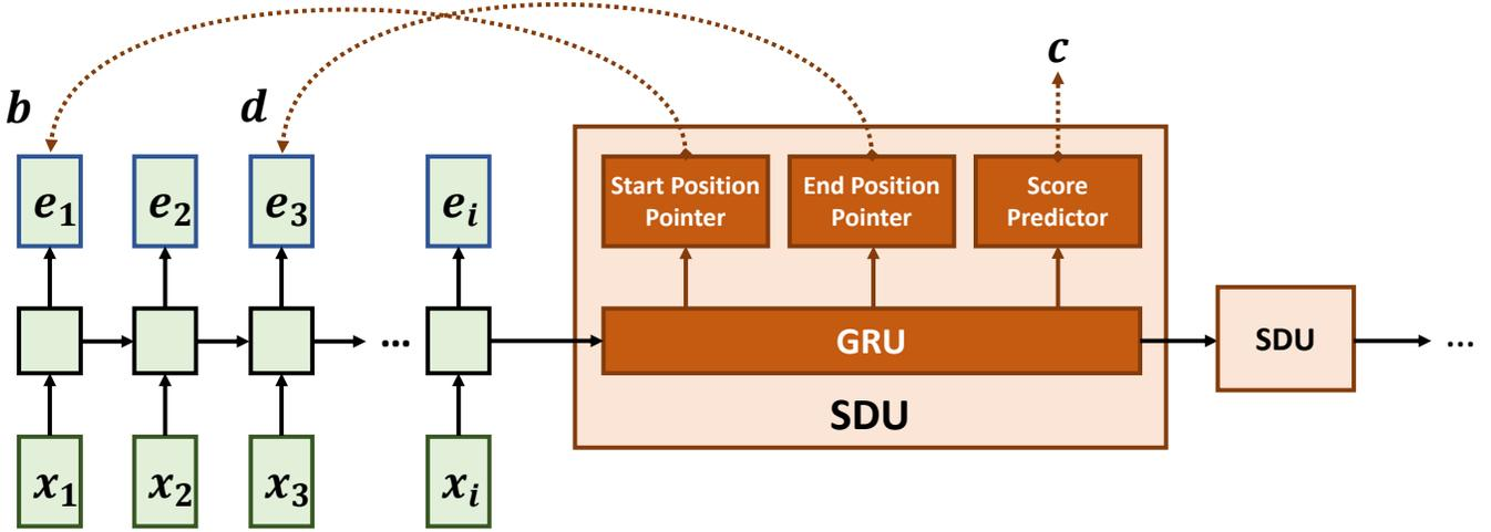
Fig. 2: An Encoder (green) processes the input sequence to create a set of encoding vectors ( $\{e_1, e_2, \dots, e_M\}$ ). At each decoding step, a Segment Detection Unit (SDU) updates the decoding state with a GRU, and based on the updated state, the SDU points to the beginning (b) and ending positions (d) with two separate pointing modules and estimates the confidence score (c) of the segment.
