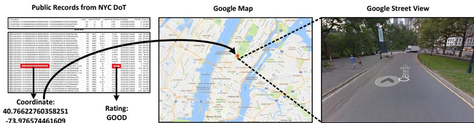
Figure 2: **Dataset creation pipeline.** We start from publicly available pavement condition rating records from New York City’s Department of Transportation. The street view corresponding to the longitude and latitude coordinates is fetched automatically via the Google Street View API and added to the dataset.
