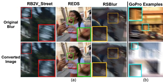
Figure 4. (a) A comparison of original images and their corresponding Blur2Blur converted version; (b) Selected examples demonstrating the GoPro dataset’s blur pattern (Zoom for best view).
