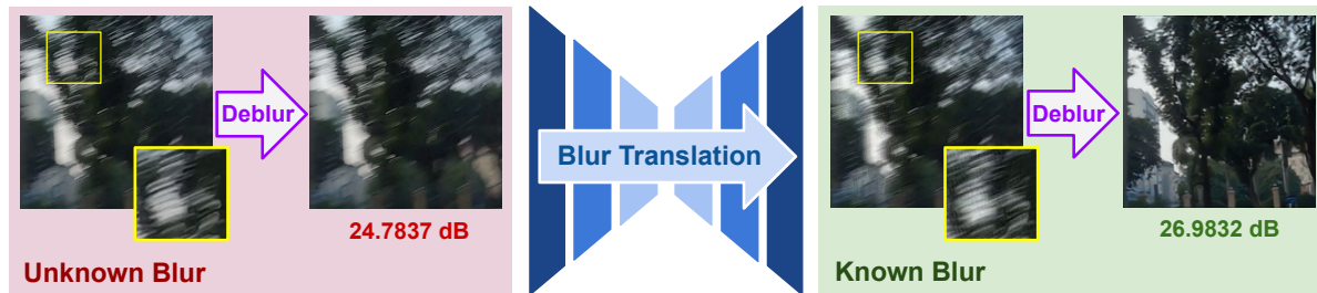
Figure 1. We address the unsupervised image deblurring problem by training a blur translator that converts an input image with unknown blur to an image with a predefined known blur. The figure shows the effectiveness of our approach. The blurry images before and after translation (left image in each box) exhibit similar visual content but have different blur patterns (zoomed-in patches). While a standard image deblurring technique fails to restore the unknown-blur image, it successfully recovers the known-blur version, yielding an approximate 2.2 dB increase in PSNR score (noted below each deblurred image on the right side of each box).
