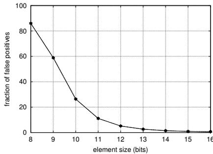
Figure 2. Effect of element and cell size parameters on the fraction of false positives
