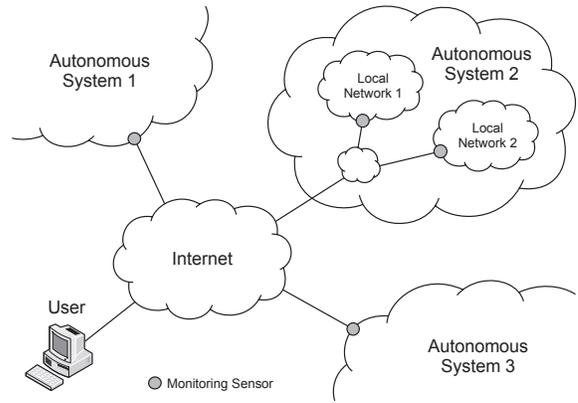
Fig. 2. A high-level view of a distributed passive network monitoring infrastructure.
