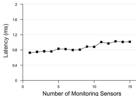
Fig. 10. Completion time for `mapi_read_results()`. This includes the processing within DiMAPI stub, the processing within each of the remote monitoring sensors, and the network round-trip time.
