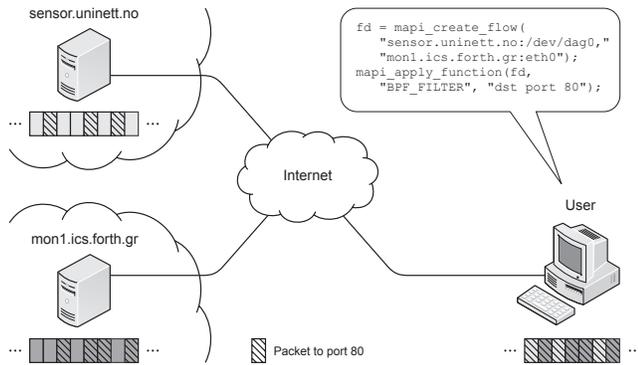
Fig. 3. An example where a monitoring application manipulates a network flow associated with two remote monitoring sensors located in different administrative domains.
