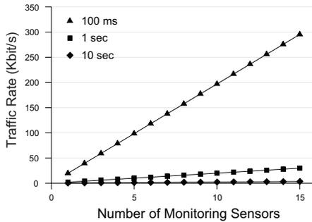
Fig. 8. Network overhead incurred with a DiMAPI monitoring application that uses function `BYTE_COUNTER`, with polling periods 0.1, 1, and 10 seconds.
