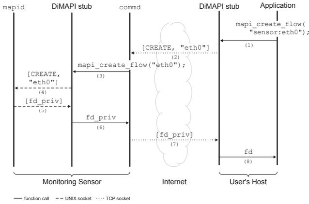
Fig. 5. Control sequence diagram for the execution of the function `mapi_create_flow()`.
