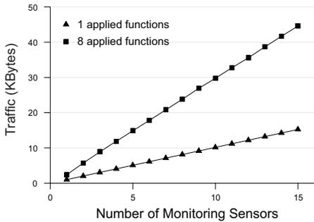
Fig. 7. Total network traffic exchanged during the initialization phase, i.e., creation, configuration, and instantiation of a network flow, when applying 1 and 8 functions.
