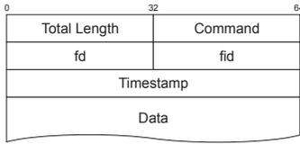
Fig. 6. Format of the control messages exchanged between the DiMAPI stub and `commd`.
