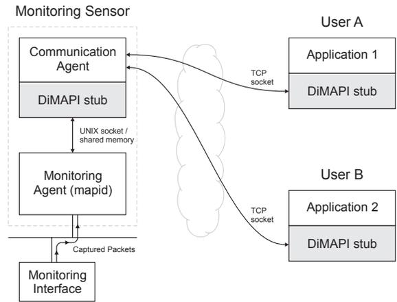
Fig. 4. Architecture of a DiMAPI monitoring sensor. Remote user applications interact with the Monitoring Agent through the Communication Agent.
