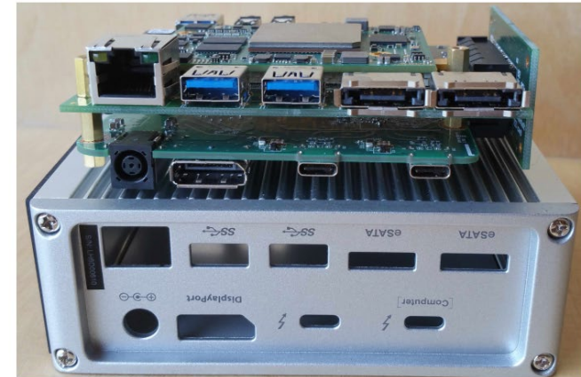
Fig. 1: Thunderbolt dock with FPGA implant, an implementation of our I/O-security research platform
