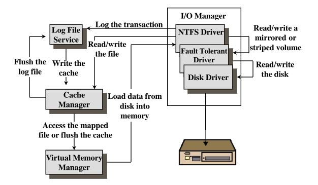
The *log file* is used to record all changes to the volume (a technique borrowed from database management) to ensure recoverability after crashes.
