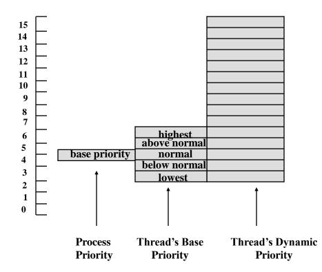
Thread's dynamic priority goes up, if thread is interrupted for I/O. It goes down if thread hogs CPU
