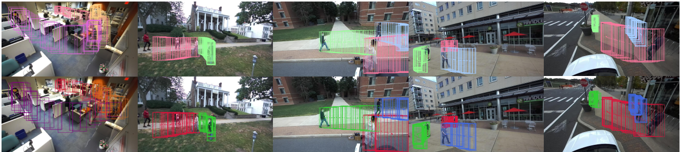
Figure 3: Samples of reconstructed vision tracklets T'_c and ground truths GT decorated in lighter (1st row) and darker colors (2nd row). Indoor scene is shown in the 1st column while outdoor scenes are displayed from the 2nd to the 5th columns. By visual comparison between T'_c and GT, ViFiT is capable of generating decent bounding boxes for missing frames.
