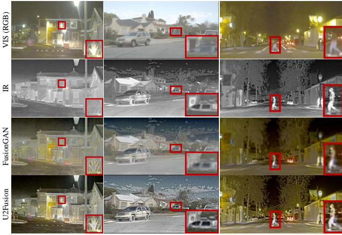
Fig. 13. Qualitative results on 3 typical VIS (RGB) and IR image pairs in the RoadScene dataset.
