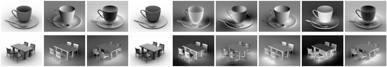
Fig. 4. The first nine harmonic images from a 3D model of one teacup (top) and a table with four chairs (bottom). The left most column contains the zeroth harmonic, the second to fourth columns contain the three first order harmonic images, and the rest are the images derived from the second harmonics (same for Figure 9). Image values are scaled to the full range of the intensity (same for Figure 9).
