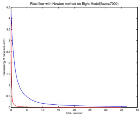
Curvature error vs. running time. Red curve Newton's method; Blue curve : gradient decent method.
