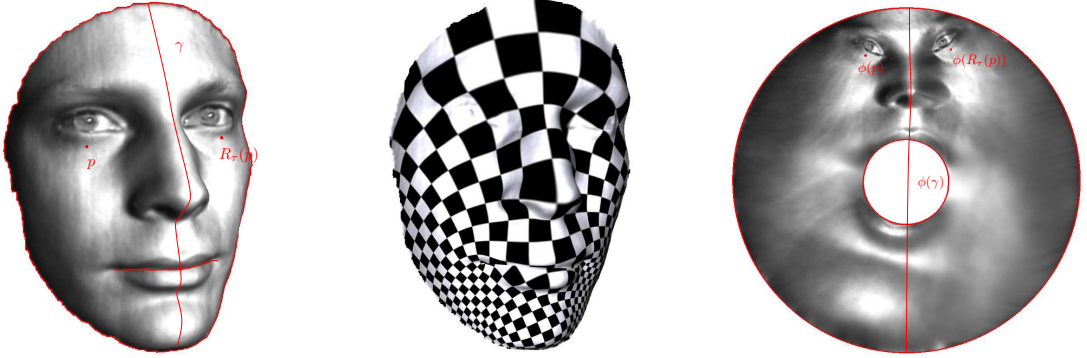
Figure 2. Conformal mapping preserving symmetry. \gamma is the intersection curve between the surface and the symmetric plane. p and R_\tau(p) are symmetric points. The symmetry is preserved on the image of the conformal mapping \phi .
