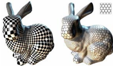
Fig. 1. The bunny surface is conformally mapped to plane, and its coordinates in plane is used as texture coordinates to pull the plane textures (check-board and tangent circles) back to the surface. Conformal mapping preserves those right angles in the left one, also maps infinitesimal circles to infinitesimal circles and keeps tangency in the right one.
