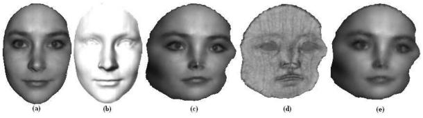
Fig. 2. Least Squares Conformal Shape Image: (a) Original surface with texture. (b) Original surface without texture. (c) Least squares conformal maps with texture. (d) Least squares conformal shape image. (e)Least squares conformal maps of the same surface, subsampled by a factor of 4, still very similar to (c).
