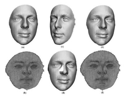
Fig. 4. An example of surface matching with holes : (a) A frontal 3D scan. (b) The LSCSI of (a). (c) A side 3D scan of the same subject as in (a), which has a hole illustrated in (d). (e) The same surface of (c,d) after hole filling. (f) The LSCSI of (e).
