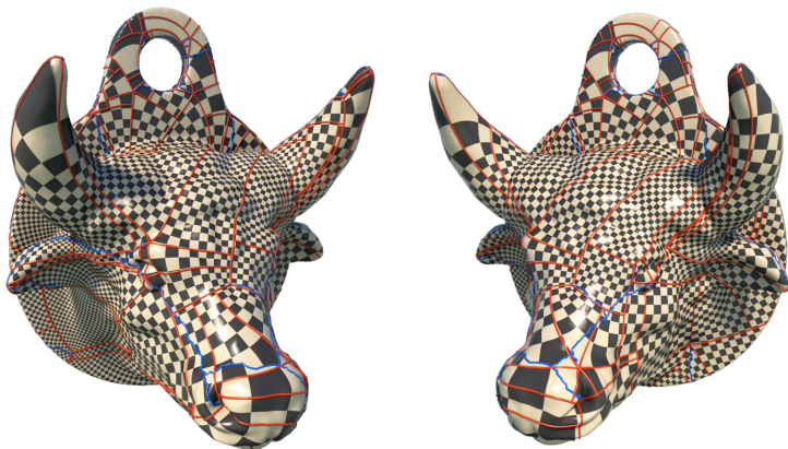
Figure: Step 2. Compute the flat cone metric using surface Ricci flow, and compute the motorcycle graph.
