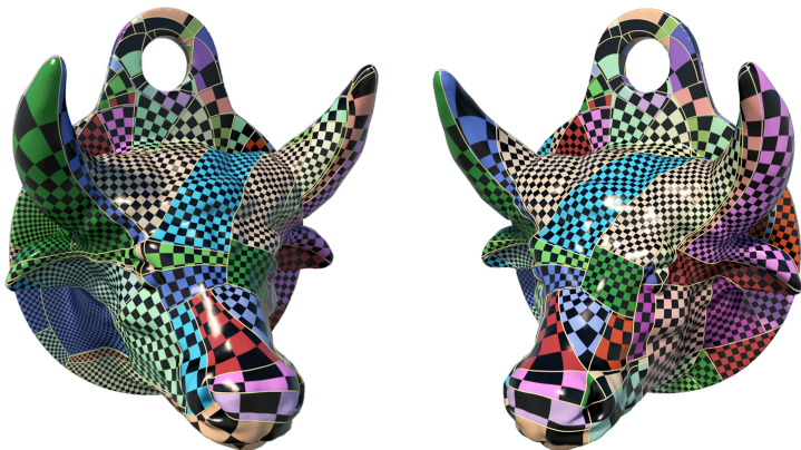
Figure: Step 4. Construct quad-meshes on each patch, with consistent boundary condition and adjust the width and the height of each quadrilateral.
