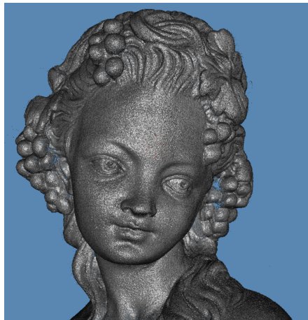
Figure: Normal estimation for merged point clouds.
