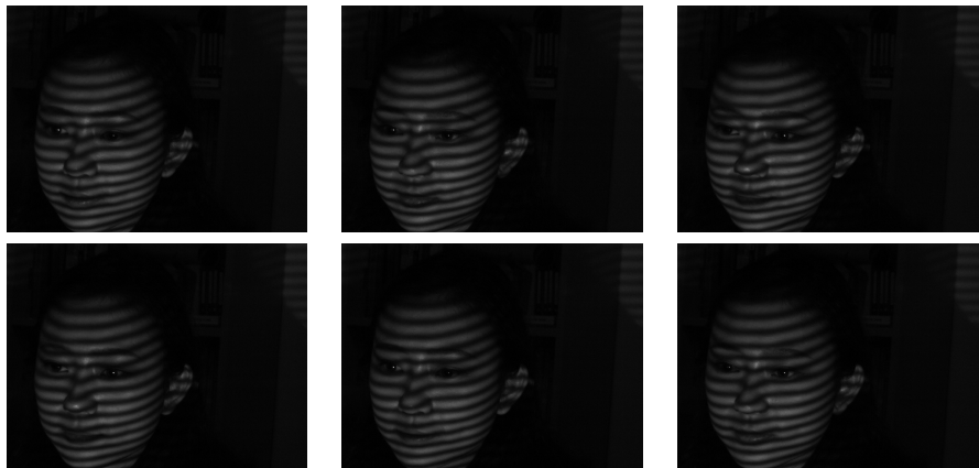
Figure: double wavelength phase shifting fringe images.
