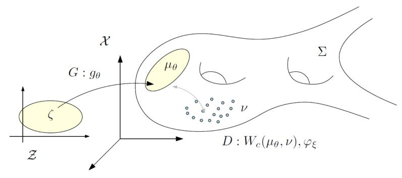
*v*-training data distribution;  $\zeta$ -uniform distribution;  $\mu_{\theta} = g_{\theta \#} \zeta$ -generated distribution; *G* - generator computes  $g_{\theta}$ ; *D* -discriminator, measures the distance between *v* and  $\mu_{\theta}$ ,  $W_c(\mu_{\theta}, v)$ .
