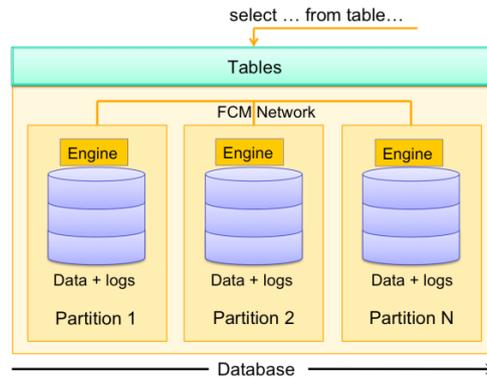
**Fig. 5.** Partitioning based parallel database architecture
