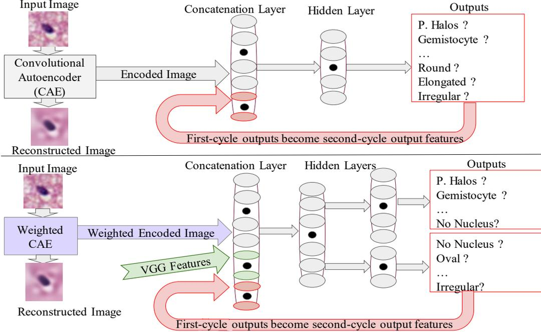
Figure 3: (Top) The Default-CNN used in [8]. (Bottom) The WFM-CNN, which uses the weighted CAE loss function, merged single and multi-label losses and pre-extracted features.
