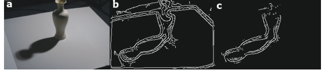
Figure 2. Shadow borders: a) original image, b) estimate using only 2D cues, c) refined estimate after first iteration
