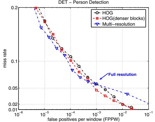
Figure 3. Comparison between HOG and multi-resolution methods using Detection Error Trade-off curves. ‘HOG’: results using original settings; ‘HOG(denser blocks)’: results using our settings in full resolution with more densely sampled blocks; ‘Multi-resolution’: results from multi-resolution. The blue arrow shows the point where we start using full resolution.
